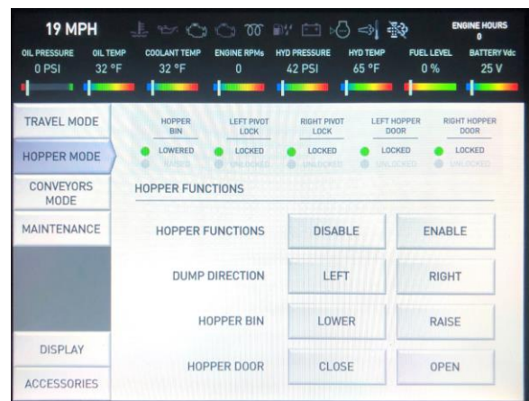
Operator Touchscreen Control Panel for Machine Operation and For Maintenance
